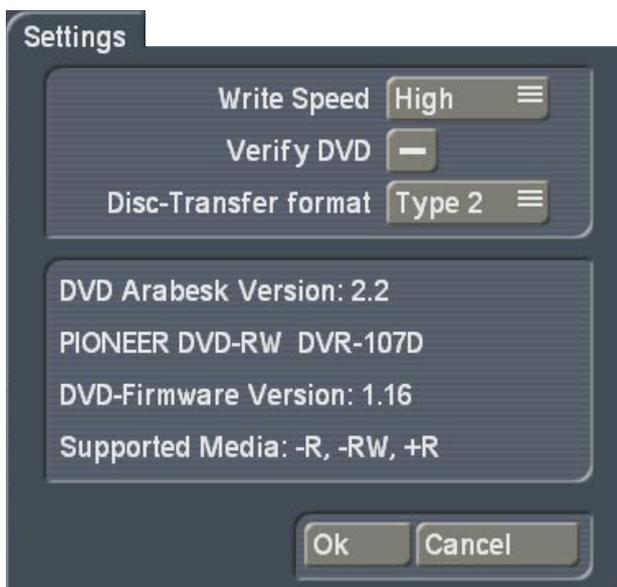
On the right next to "Disk-Transfer Format", you must now select DV "Type 1" or "Type 2" as the AVI file type for the DV Direct video footage:
